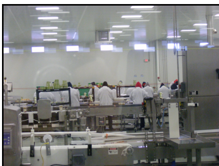
▲ Cold Area Food Preparation at Sheetz Kitchen Facility. Room temperature is 36 to 38 degrees F.
